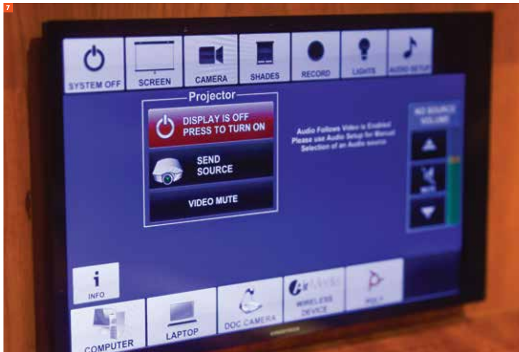
[7] The room is controlled through a touchscreen panel, the same type and interface as in classrooms across the University.
